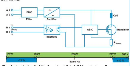
The electronic circuit of the Sprecher + Schuh CA6 contactors allows a very wide operating voltage with precise opening and closing levels. The design includes EMC filters and a built-in PLC interface.
