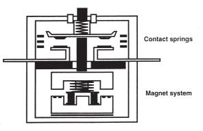
Principle design of a contactor
