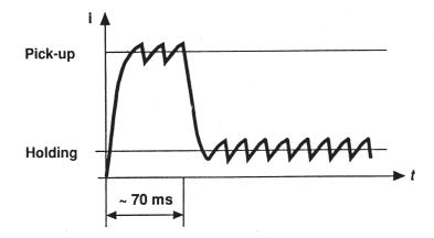
Pick-up and hold-in current with electronic control
